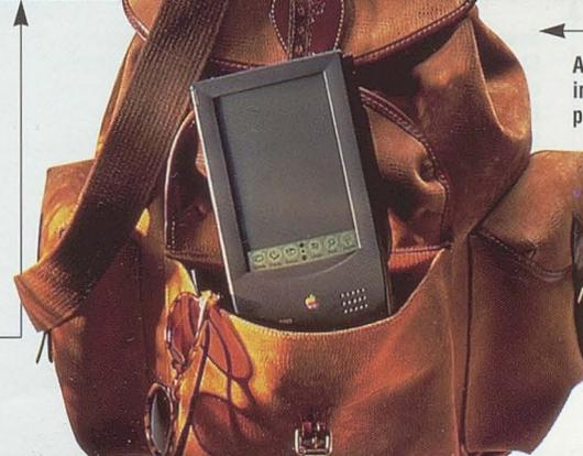
Apple Computer introduces the handheld personal computer, Newton MessagePad, hyping it as technology for "the new mobile society." The electronic diary can send faxes and turn handwritten notes into printed messages.
