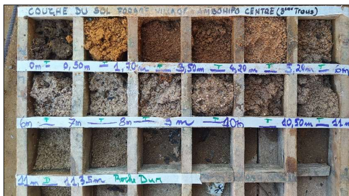
Soil samples taken during drilling at Ambohipo Centre; the third drilling attempt was successful
