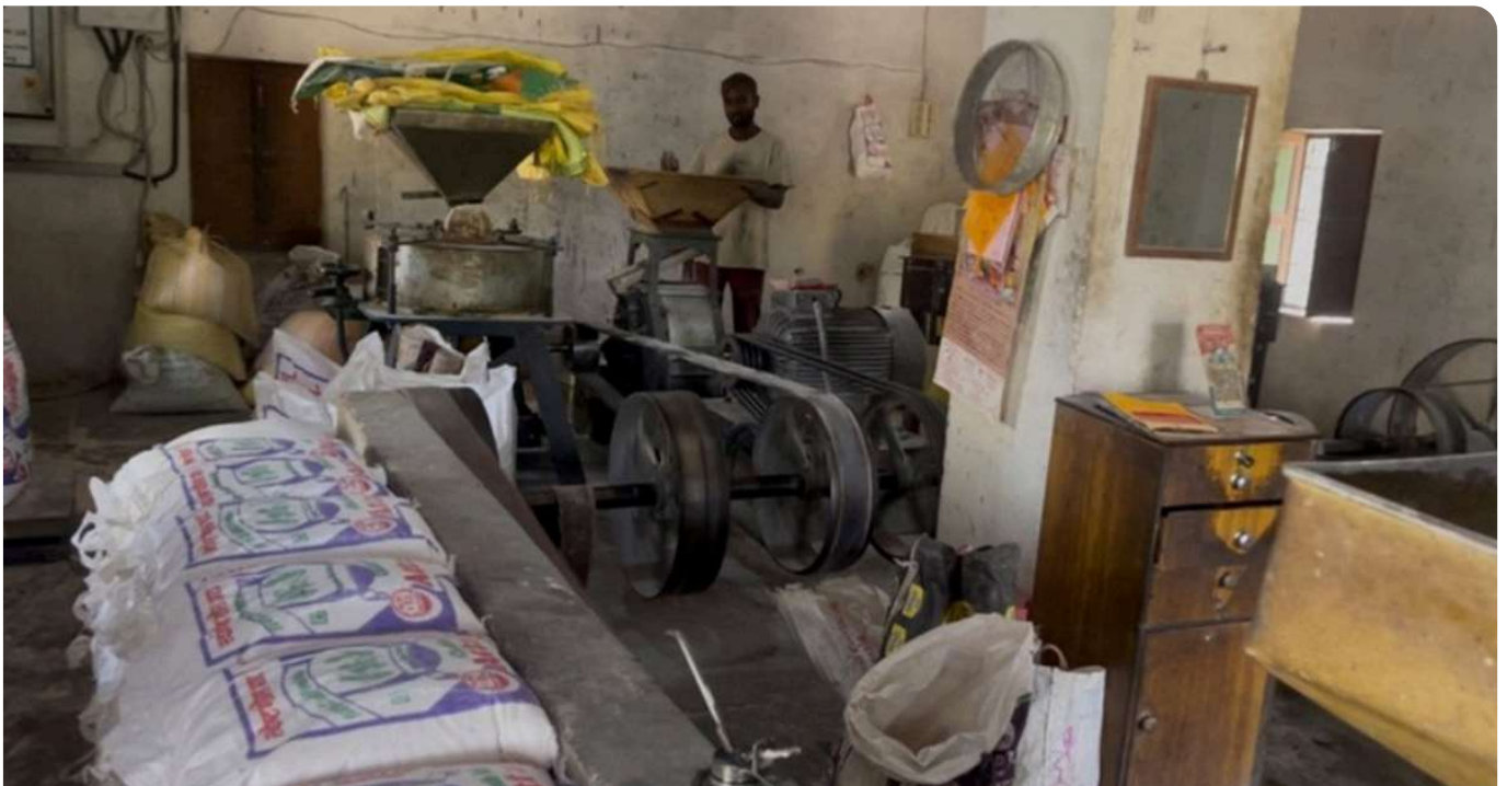
The traditional atta chakkis that are powered by diesel make immense noise that can cause hearing problems
