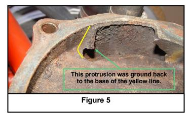
Because of the location of the volute opening, you are not likely to notice the casting protrusion unless you were specifically looking for it.
