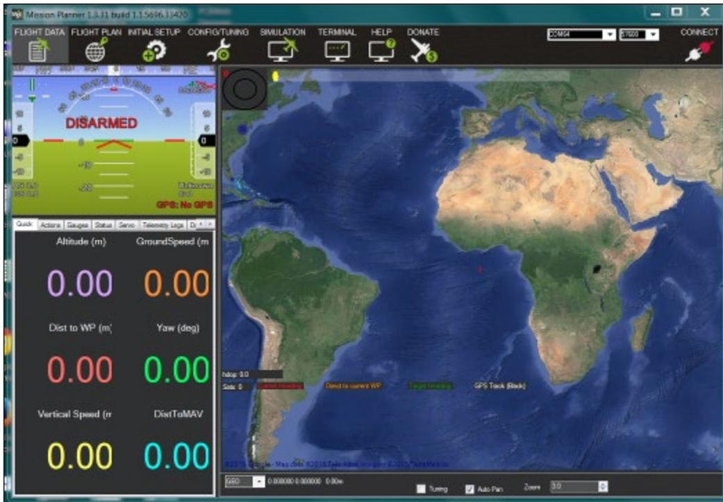
This is the basic screen. You'll then need to configure your radio's COM port and then press the **CONNECT** button in the corner on the upper right-hand side of the screen. As you move the quadcopter around, you will see the measurements change. If you are having problems connecting to the Pixhawk, there is a lot of help available on the website.
