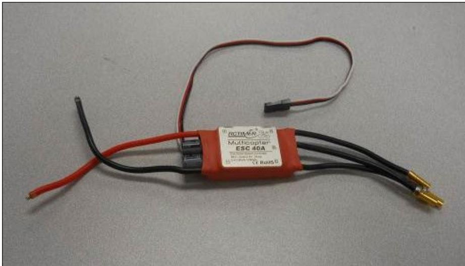
The red and black wire connectors are the connectors that are soldered to the bottom plate of the frame. The other three connectors will connect to the motor.
