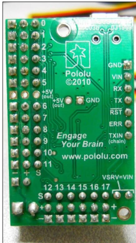
Now you need to connect the servo motor controller to your battery. For this project, you can use a 2S RC LiPo battery. The 2S means that the battery will have two cells, with an output voltage of 7.2 volts. It will supply the voltage and current needed by your servos, which can be in the order of 2 amps, as shown in the following image:
