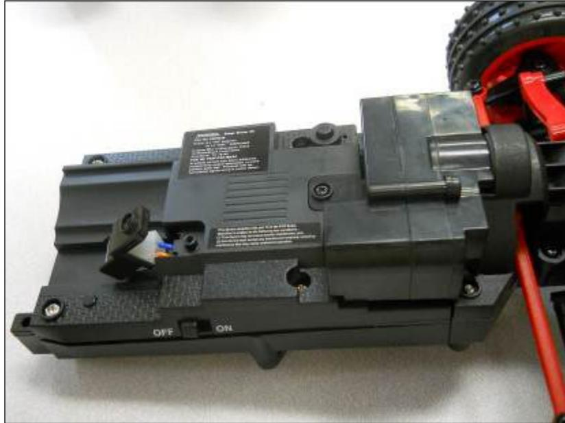
Remove this plug and these wires; you'll use Raspberry Pi Zero and a motor controller to provide the voltage to the drive system of the car. The motor will run faster or slower based on the voltage that is applied to these wires and the polarity of the voltage will determine the direction. Raspberry Pi Zero will need to provide a positive or negative 6-volt signal to control the speed and direction of the car.
