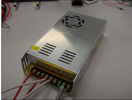
The connections on the power supply are clearly marked; you'll connect the 6-volt power supply and GND connections to the connections marked BAT on the servo controller.
