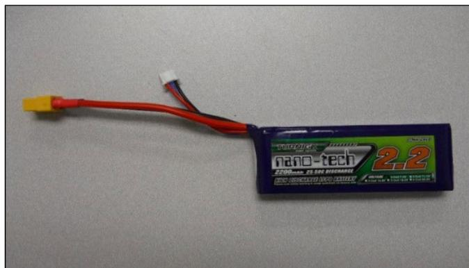
This battery will come with two connectors, one with larger gauge wires for normal usage and a smaller connector to connect to the battery recharger. You'll want to build connectors that can connect to the screw-type connectors of the servo controller. I purchased a few XT60 connector pairs and soldered some wires to the mating connector of the battery and then screwed these into the servo controller.
