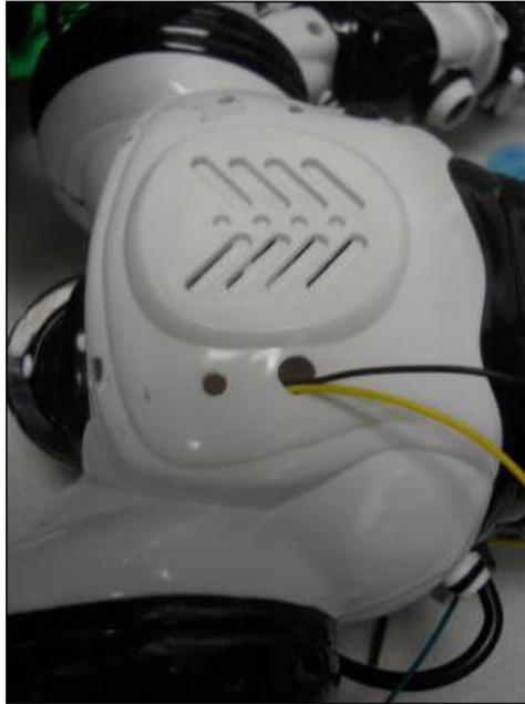
5. This picture also shows two more holes on either side of the shell, which you can use together with cable ties to attach the Raspberry Pi to the robot. Now you can put the shell back onto the robot.
