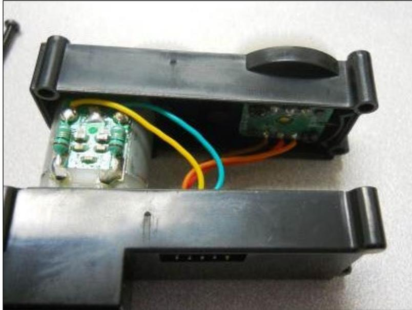
As you can see in the preceding image, the blue and yellow wires are attached to a DC motor, and the orange, brown, and red wires are attached to another control circuit. The motor will drive the wheels left or right, the polarity of the voltage will determine the direction, and its magnitude will cause the wheels to turn more or less sharply. The orange, brown, and red wires are interesting, as their purpose is a bit difficult to discover.
