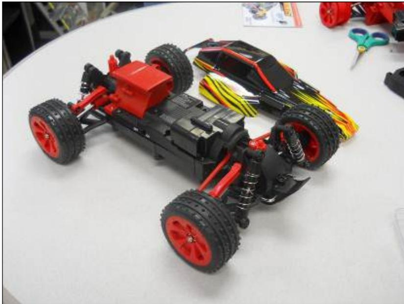
There are two connections that you will want direct access to. The first is the drive motor, and the second is the steering mechanism. For this particular model of RC car, the drive mechanism is in the rear. What you are normally looking for is two wires that will directly drive the DC motor of the car. In this system, there is a connector in the rear of the car; it looks similar to the following image:
