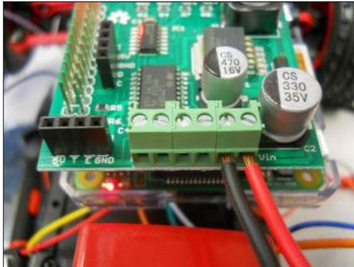
2. Next, connect the rear drive signal to the motor 1 connectors on the board, as in the following image:
