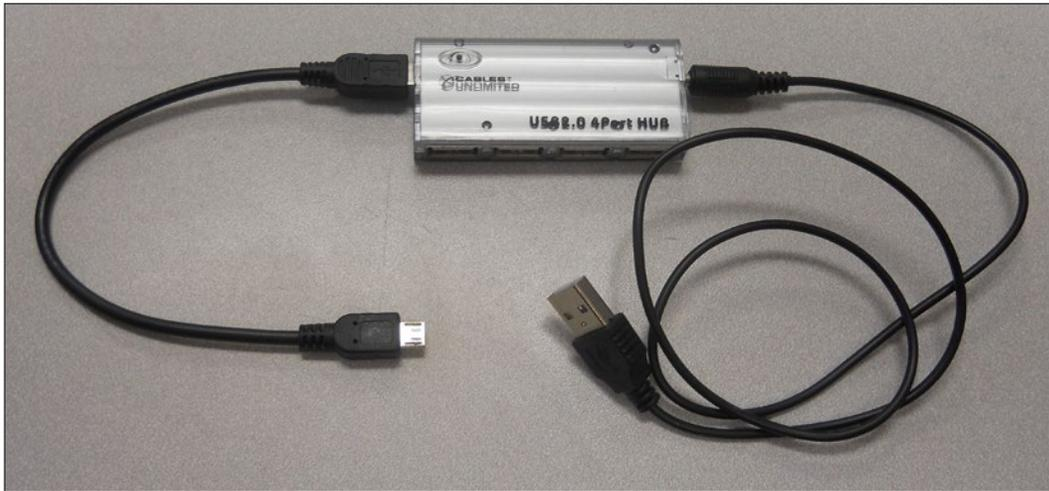
Note that there are two connections on this hub. The one to the far right is a power connection and it will be plugged into a battery or a USB power adapter with a USB port. The connection to the left is the USB connection, which will be plugged into the Raspberry Pi. To connect the power USB board to the Raspberry Pi Zero you need a cable that connects to a microUSB connector. Now, you'll have more connections to add a mouse and keyboard, webcams, and a USB WLAN device.
