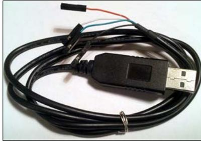
A USB to TTL serial console cable
