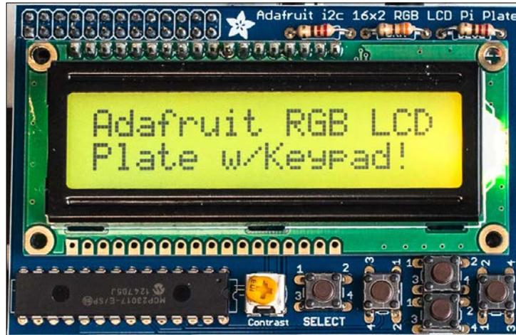
Adafruit I<sup>2</sup>C 16x2 RGB LCD Pi Plate with keypad buttons
