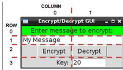
Grid layout for the Encrypt/Decrypt GUI
