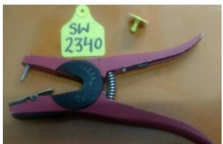
Figure 1: Ear Tagging Machine with Plastic Ear Tag
