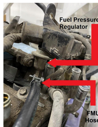
Figure 4: Fuel Pressure Regulator (Outerport Hose)
