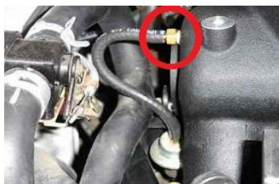
Figure 5: Boost Reference Source (Backside of Supercharger)
