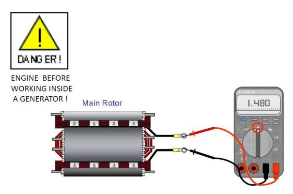
The Main Rotor resistance is checked with a multi-meter set on the  $\Omega$  range. Disconnect the main rotor leads from the rotating rectifier mark (+) and (-). Measure windings for a short or open. Record resistance reading and compare value to resistance chart.
