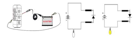
A good rectifier will light the test light in only one direction. It should not light the test Light when the leads are reversed.. A faulty diode inside the full wave recifier if it lights The test light in both the directions (short circuit diode) or no light in either direction (open circuit diode).
