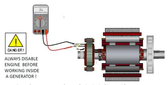
The exciter armature resistance is checked with a multi-meter set on the  $\Omega$  range. Disconnect the exciter armature leads(AC1, AC2 & AC3) from the rotating rectifier. Measure windings for a short or open. Record resistance reading and compare value to resistance chart.
