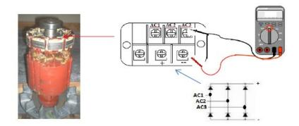
The Rotating Rectifier is a Full Wave Diode Bridge Rectifier and utilizes four (6) diodes to convert one full wave of alternating current into one full pulse of direct current.
