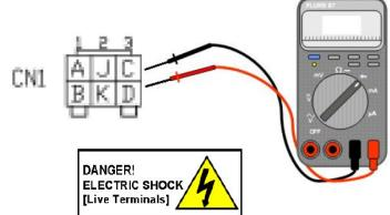
The no load voltage should be: (Back probe CN1 connector. See Chart for specifications per model)
