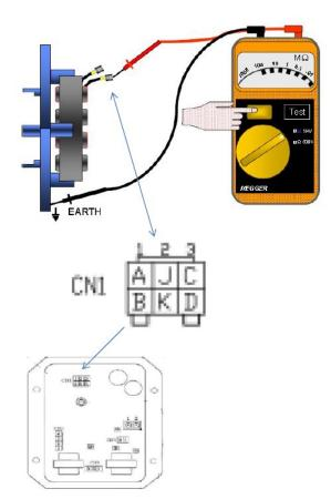
Disconnect the 6 – pin connector from the AVR.
