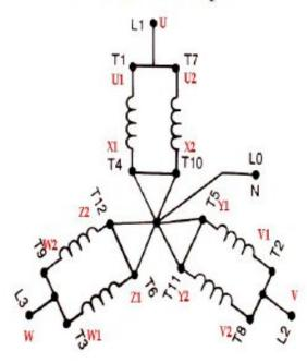
Parallel connection produces lower voltage and higher amperage.
