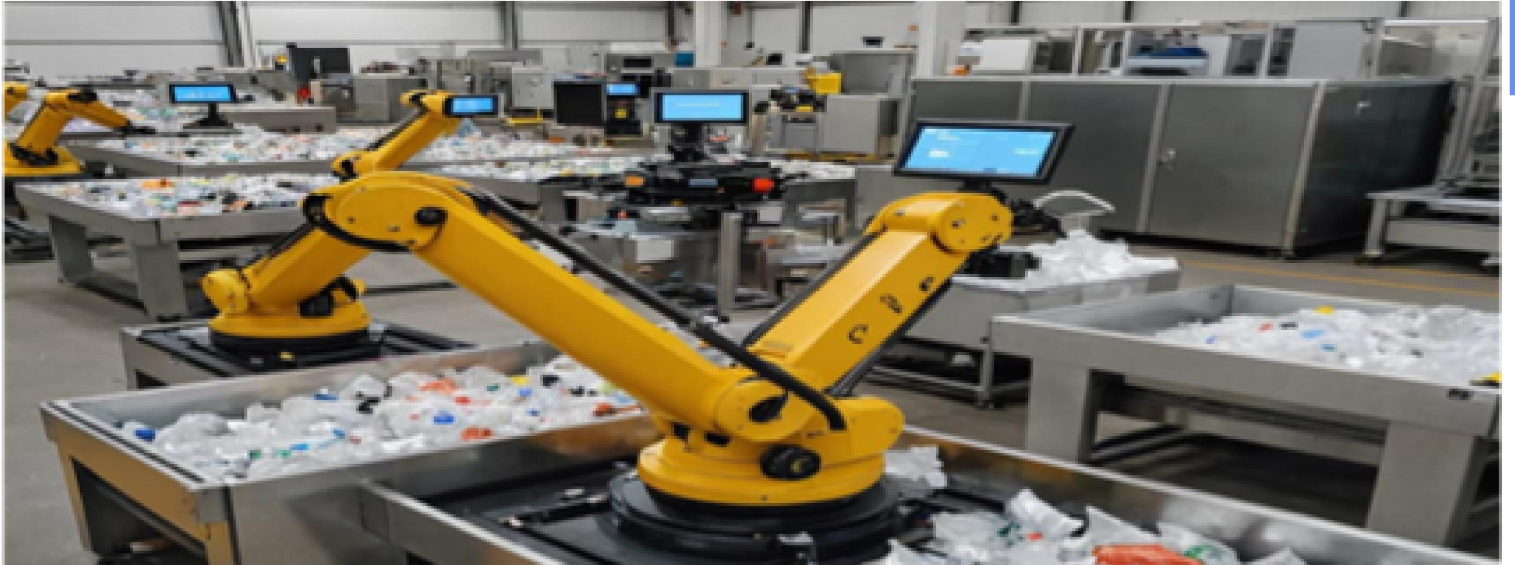
Redam is a platform that helps to classify recyclable waste for contamination and recycling by using an AI robot arm that has learned an object recognition model based on machine learning.
