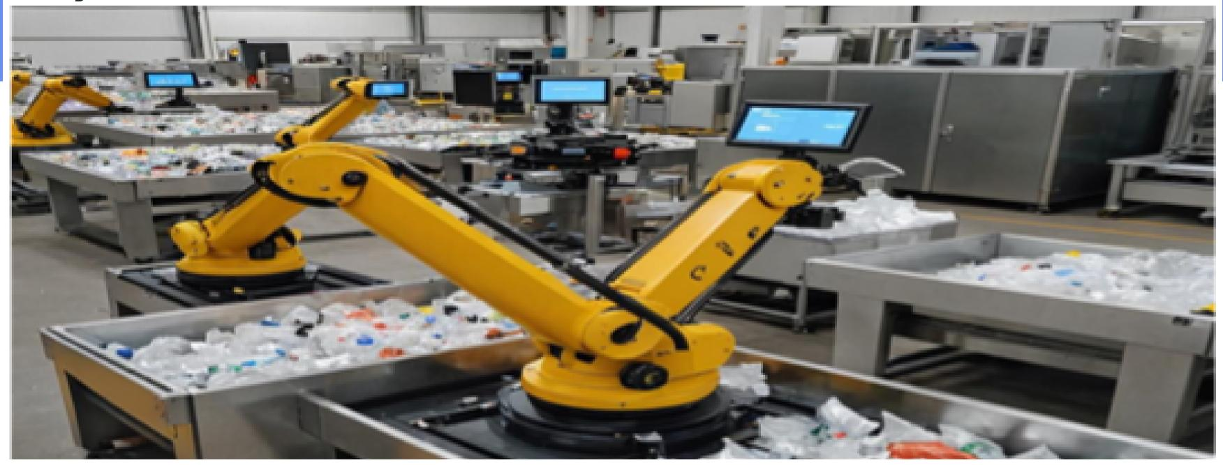
Redam is a platform that helps to classify recyclable waste for contamination and recycling by using an AI robot arm that has learned an object recognition model based on machine learning.
