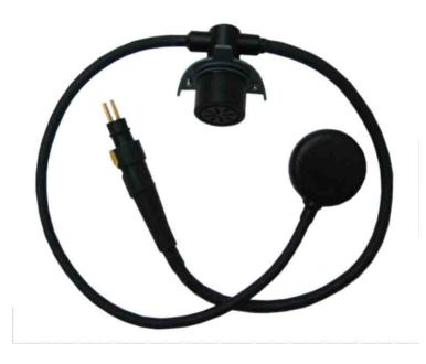
The AGA Comms Assembly is comprised of a dynamic Hi-Sense microphone with cover plate and a fully encapsulated earphone, all connected to the surface operator via a wet mateable connector. The assembly is easily fitted to the FFM using the made-to-measure cover plate which creates a seal when secured with the two supplied mount screws.
