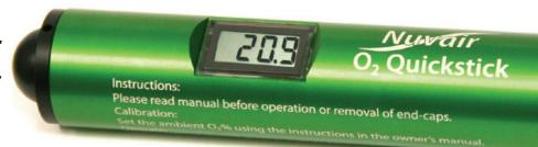
The Nuvair  $O_2$  Quickstick is the first diver-friendly oxygen analyzer available anywhere! Easy to use, effective, rugged and amazingly affordable, it is equally convenient for non-divers who need a quick and reliable oxygen analysis above water. The  $O_2$  Quickstick is designed for anyone who wants the security and convenience of having their own oxygen analyzer without having to pay a small fortune to own one.
