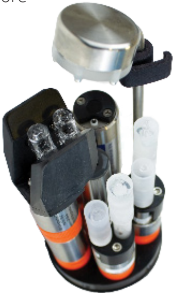
Streetlamp UV installed on AML-6
