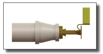
Do not remove the sprinkler strap until the sprinkler system is under commissioning for operation.
