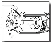
The Horizontal Sidewall Sprinkler must be installed with the centerline of the waterway horizontal and perpendicular to a back wall surface. It is recommended that a lightweight spirit level be used to level the sprinkler fitting prior to installing the sprinkler. Using a square ensure the perpendicularity of the waterway centerline to the mounting surface.
