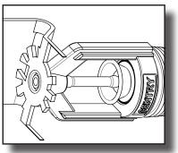
The Horizontal Sidewall Sprinkler must be installed with the centerline of the waterway horizontal and perpendicular to a back wall surface. It is recommended that a lightweight spirit level be used to level the sprinkler fitting prior to installing the sprinkler. Using a square ensure the perpendicularity of the waterway centerline to the mounting surface.
