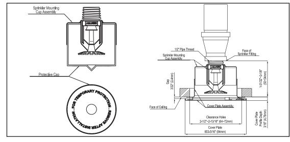
Properly installed sprinklers must have a nominal 3/32" (2.4mm) air gap between the lip of Cover Plate and the ceiling. The air gap is necessary for the proper operation of the sprinkler. If the ceiling is to be painted after installation of the Cover Plate Assembly, care must be taken to ensure that new paint does NOT seal off the nominal 3/32" (2.4mm) air gap.
