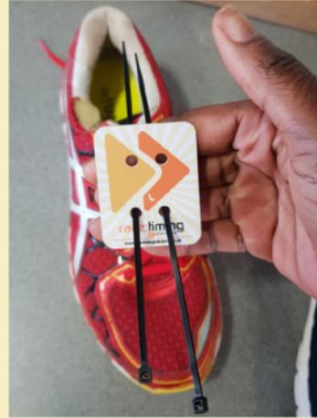
thread the cable tie through the holes on the chip
