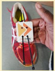
thread the cable tie through the holes on the chip
