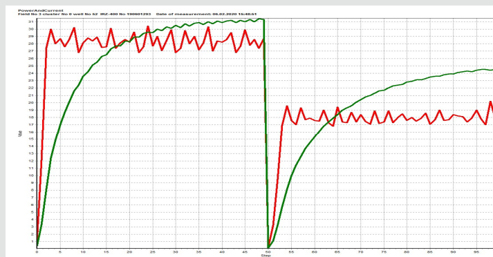
Power consumption and current vs piston position
