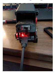
Remove the slip on the ring on the back. Once removed, you can now lift out the main carriage, make sure to line the battery back up with its slot when reinserting! On the exposed bottom of the carriage are 2 usb ports, one on the blue board and one on the black esp32. Connect to the blue tp4056 to charge, if you so desire to reprogram, plug in to the esp32 and insert the usb cable to your computer.
