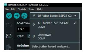
The board will be the ESP32-C3 dev board, or for me it ended up being DFRobot beetle ESP32-C3
