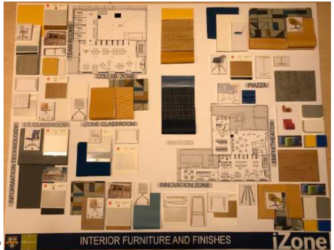
Interior Finishes Board presented to the client to display final material swatches and their adjacencies
