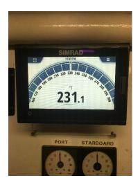
A client got in touch detailing that an analogue Simrad AR80 type Gyro repeater installed at an emergency steering position had stopped operating correctly. AMEA Services were able to attend and verify with a NMEA0183 reader that it was indeed the Gyro repeater and not the signal that was the issue.
