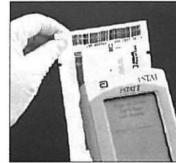
Remove cartridge from pouch. Handle the cartridge by its edges. Avoid touching the contact pads or exerting pressure over the center of the cartridge.
