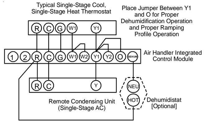
**Figure 9 - Typical Single-Stage Cooling with Single-Stage Heating**
