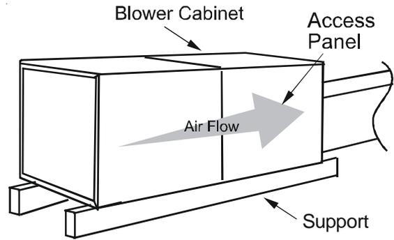
Figure 4 - Attic Installation
