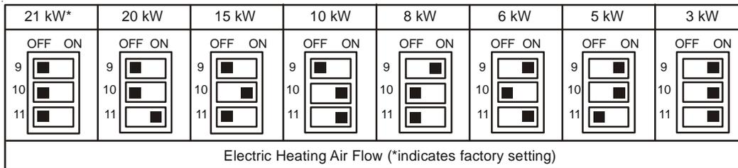
Figure 20 - Dip Switches
