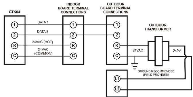
**Figure 23 - System Wiring**
