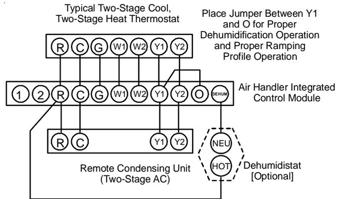
**Figure 10 - Typical Two-Stage Cooling with Two Stage Heating**
