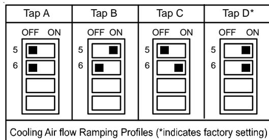
Figure 15 - Switch Positions and Taps
