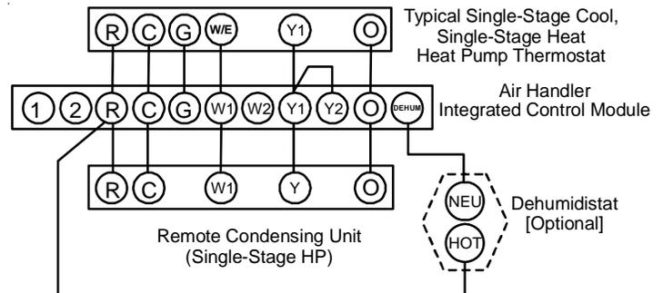
**Figure 11 - Typical Single-Stage Heat Pump with Auxiliary/Emergency Heating**
