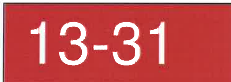
Runway Hold Sign
