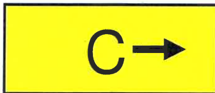
Runway Exit Sign
