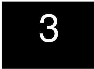
Runway Distance Remaining Signs
