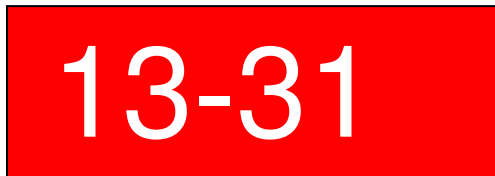
Runway Hold Sign
