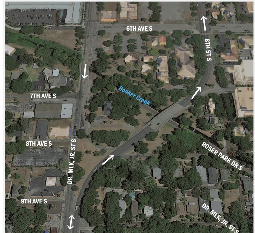
*Two-way conversion provides an opportunity to re-purpose underutilized land, especially at the north and south ends of the pairs that are connected with diagonal roadways.*
