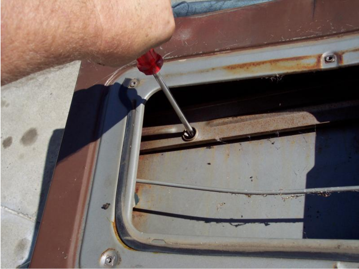
Remove the two door handle screws. One is on the inside of the door panel..
