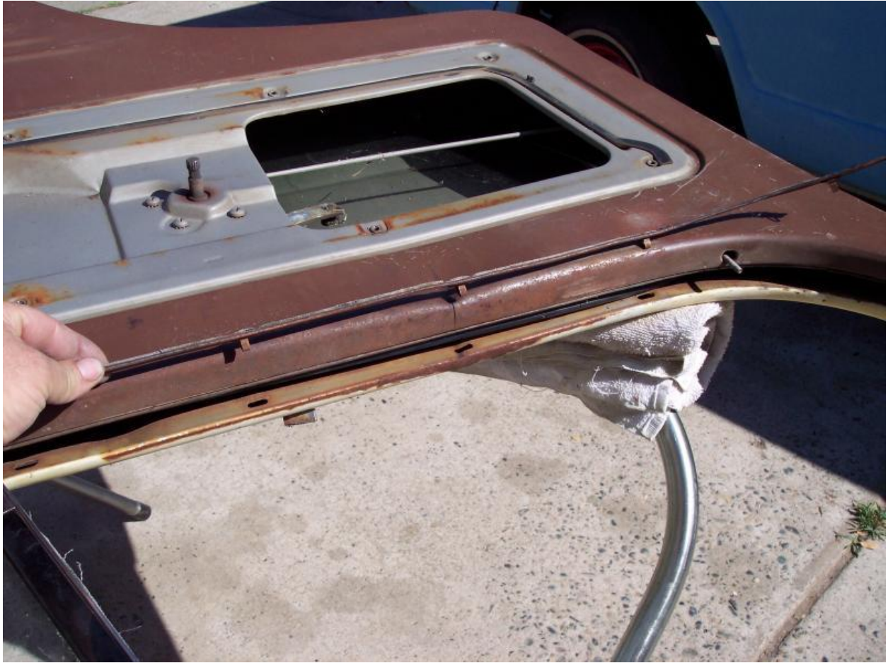
This shows the seal removed and the clips that hold it to the door.
