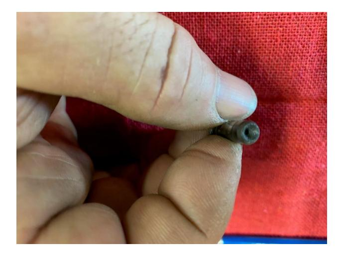
Once the pin is almost out, it should be removable by hand. Once the pin is out, pull the lever out while cupping your hand below the removed pin area. Sometimes, there was a small wave washer installed on the lower pin area. Check for this washer or pieces of what's left of it.
