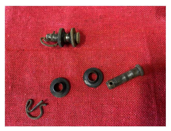
The pic below shows a new bushing next to an old one. The new bushing is much more squared off and will result in much less looseness. I'm having trouble locating these bushings, any help is appreciated. There was a couple of Hurst Shift Arm Bushing Pit Pack kits available but they didn't fit the 1<sup>st</sup> gen shift arm I was working on. I'm looking for replacement bushings.
