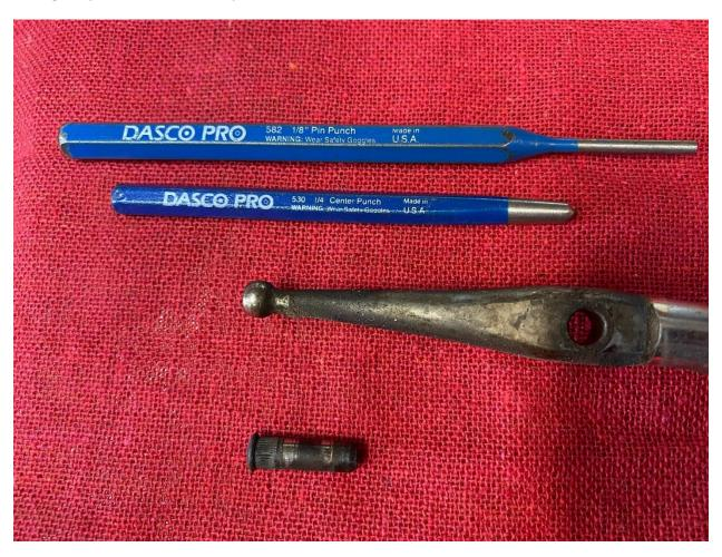
Below is a view of the bottom of the pin. Note how a pointed punch will fit nicely in the base.
