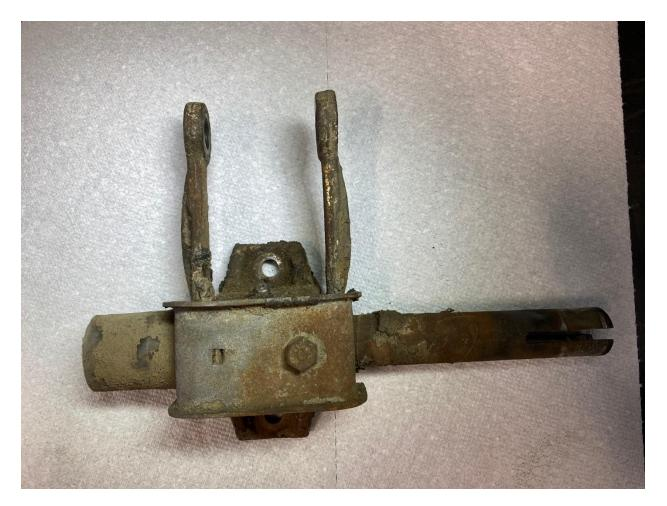
The pic below shows the 2<sup>nd</sup> Gen VCVs shift mechanism. The 2<sup>nd</sup> gens have a flat spot on the main body that (I believe) is intended for a grease fitting but I have never seen one installed from the factory. It comes from the factory not even drilled or tapped for a fitting. (WTH!) If you have opportunity to remove one, I advise installing a grease fitting as shown.
