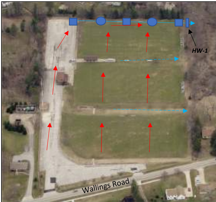
Eagleview (CEGIS) of Heasley Soccer Fields PPN#489-19-010, with approximate catch basin locations and general flow direction. April 4, 2019
