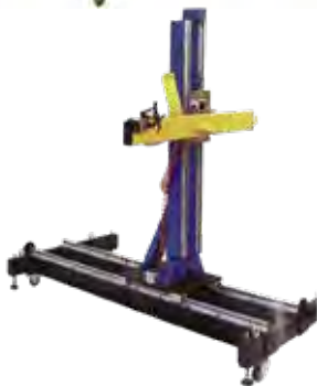
TUBE-TO-TUBESHEET POSITIONER (pneumatic) With the tube-to-tubesheet positioner, the RBK 60 S can easily be positioned without a balancer and centred pneumatically with the lever on the positioner. The head is aligned with a matching centring on the tubesheet. The positioner stands on castors and is fixed in front of the tubesheet with a screw adjustment.
