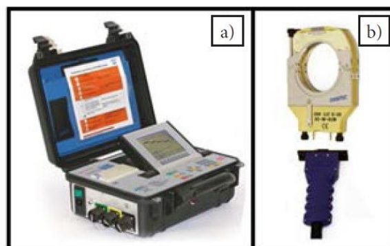
Fig. 4. Components of the orbital welding station: A- controller, B- closed welding head
