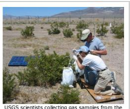
USGS scientists collecting gas samples from the unsaturated zone. Subsurface gases are drawn through a small glass tube filled with an adsorbing material, which traps mercury or volatile organic compounds for later analysis.
