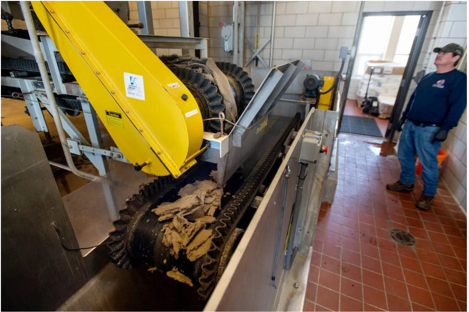
Biosolids are moved along a conveyor and sent down a shoot into a container below. Credit: Linda Coan O'Kresik / BDN
