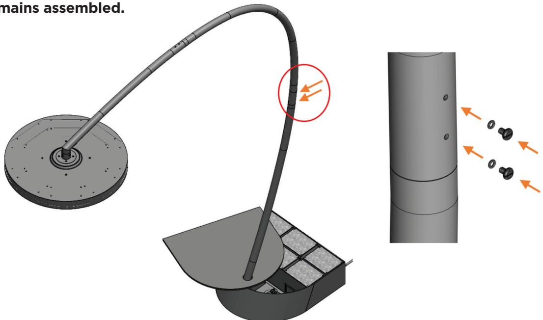
25. Using a spirit level and phillips head screwdriver, adjust the angle of the heater head to be level by adjusting the 4 x Dome Head screws (M4 - Length: 6mm) on the heater head.
