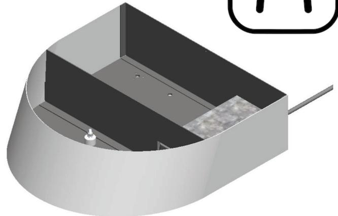
6. **NOTE:** If installing in areas subject to high winds, gusts or hurricanes, heater base must be bolted down to ground using appropriately sized and type bolts (not included) suited for the ground surface through the 5 X Holes in the Heater Base.
