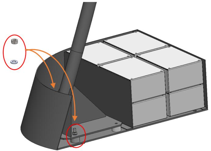
11. Fasten the **rear** two slots of the Lower Arm section to the Base using 2 X M8 Washers, and 2X M8 - Length: 35mm bolts.
