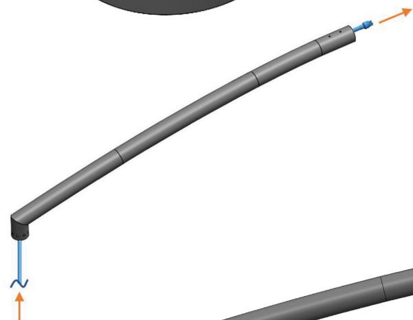
17. Attach the top arm section to the Heater Head using the 2 X Dome Head Screws (M5 - Length: 14mm) (preassembled to head).
