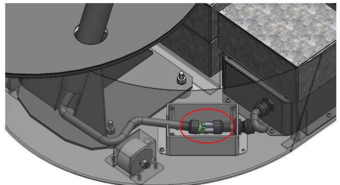
28. Attach the rubber cable grommet around the cable, and place it in the square slot in the connector box, ensuring the flat face is facing upwards.
