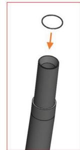
13. Unwrap the Base Cover from its packaging and confirm that seal is fitted to the arm slot.
