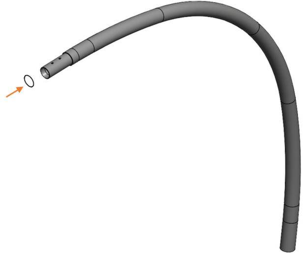
20. Check that 1 X Large O-ring (35mm ID) is fitted to the connector section of the Middle Arm.
