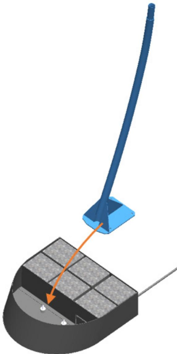
10. Fasten the **front** two slots of the Lower Arm section to the dampeners using 2 X M8 Washers, and 2X M8 Nuts.
