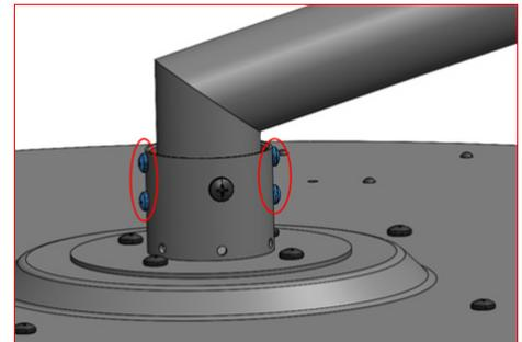
26. Within the Base, remove 4 X Oval Head screws (#4-40 - Length: 3/8") from the Small Connector Box, and remove lid.
