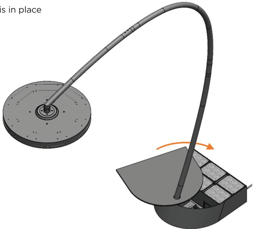
31. Fasten the Base Cover to the Base using the Dome Head Screw (M4 - Length: 6mm). This screw is packaged with the remote control inside the base.
