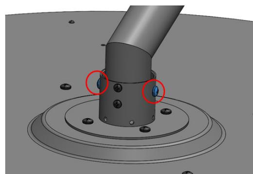
18. Fasten the 4 X Dome Head Screws (M4 - Length: 6mm) to the head to lock the angle of the Heater Head relative to the Top Arm section.
