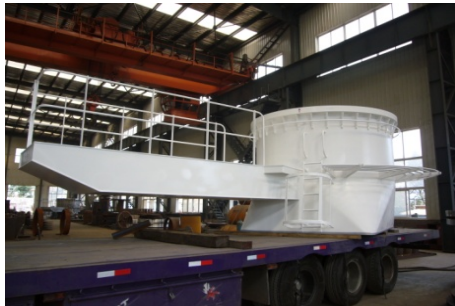
Deck crane pedestal
