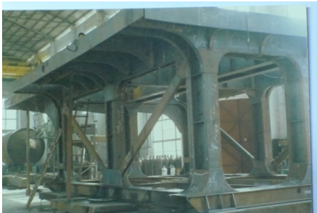
Stacker reclaimer platform
