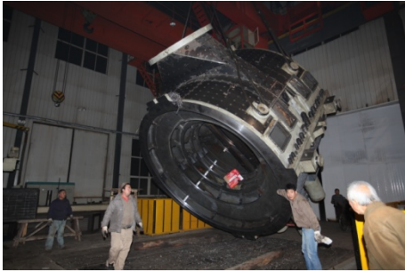
Steam turbine inner cylinder
