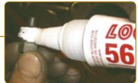
Step #2. Apply Loctite 567 PST Thread Sealant with PTFE
