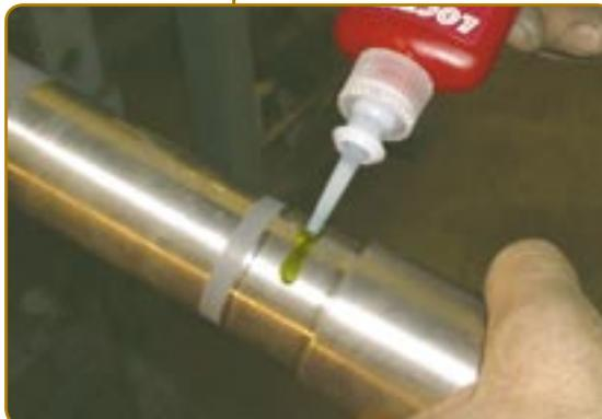
Step #2. Apply Loctite 641 Retaining Compound
