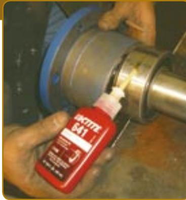
Step #2. Apply Loctite 641 Retaining Compound.
