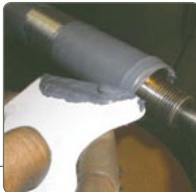
Step #4. Apply Loctite Fixmaster Superior Metal
