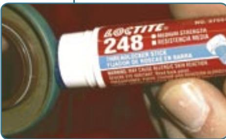
Step #2. Apply Loctite 248 Medium Strength Threadlocker Stick
