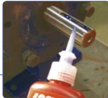
Step #2. Apply Loctite Medium Strength Threadlocker
