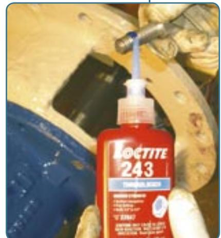
Step #2. Apply Loctite 243 Medium Strength Threadlocker.
