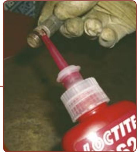
Step #2. Apply Loctite 262 High Strength Threadlocker
