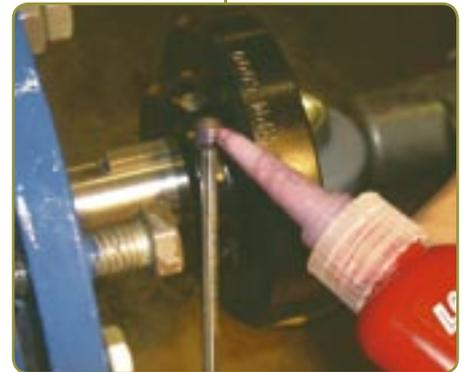
Step #3. Apply Loctite 222 Low Strength Threadlocker.
