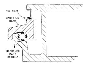
FIGURE 1 - CAST IRON DRIVE WITH INSERTED RACEWAY BEARING
