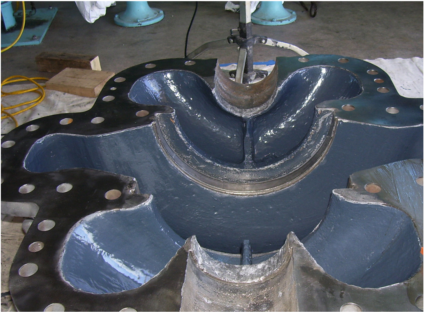
Figure 2. Pump interior after coating with brushable ceramic epoxy
