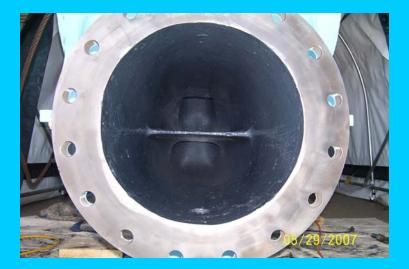
Echo Post Interior Coating vs. Post Mechanical Refurbishment Performance Comparison Increase 10' of Head, Increase of 5% Efficiency Total Efficiency Increase from Mechanical & Coating 8.2%
