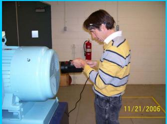
600 HP, 18x16 Bottom Suction HSC Pump, Installed 1990, Pre Rebuild/Pre Coating Performance Analysis (25' Loss of Head, 10% loss of Efficiency)
