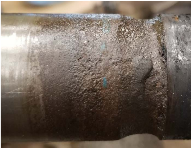
Severe packing damage
