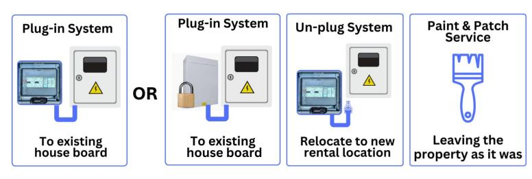
The options include a weatherproof or lockable Plug-in System for extra security as well as locating the system inside the home when a landlord purchases the system.
