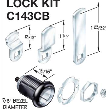
**Application** – Universal type lock for either doors or drawers. Kit will accommodate most locking applications for material thickness 1/16" – 1/2".
