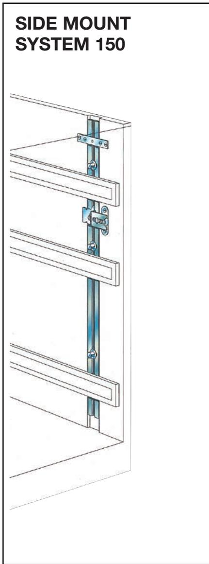
LOCK BAR MUST BE RESTRAINED FROM DROPPING WHEN IN OPEN POSITION
