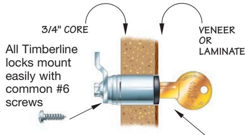
All Timberline locks consist of two separate components: a Lock Plug, and a Cylinder Body. A Change Tool (D500KY, see page 7) is required to remove lock plugs from the cylinder bodies.
