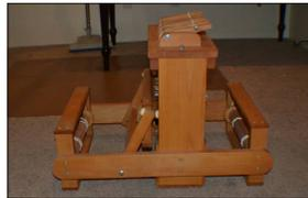
**AVL loom.** 16 harnesses and only 2 treadles since it is a dobby loom. The dobby takes all the note taking out of the process by using pegs to make the treadling work. You only step on one treadle to raise the harnesses and the other one to lower them and advance the dobby pegs. It has an integral seat, cloth advance, sectional and plain beams and the AVL tension box track. \$4,000 orOBO. Made from rock maple.
