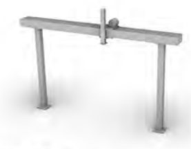
Linear Robot Cartesian Coordinate System. Limited workspace, modular, expandable. Used for moderate to heavy payloads.
