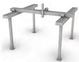
Gantry Robot Cartesian Coordinate System. Heavy-duty, modular, expandable. Used for heavy payloads.
