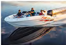
Case Study 2: 17' Tahoe open skiff. Thermwood Corporation. 2018. Dual gantry Large Scale Additive Manufacturing (LSAM). Extruded thermoplastic CNC milled plug mould.
