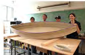
Case Study 1: 7' Flat-bottomed canoe. University of Washington Fabbers Club. 2012. Single gantry extruded recycled thermoplastic. Extruded HDPE manufacturing demonstration project.
