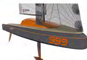
Case Study 5: 21' Livra 6.50 racing yacht. Urea Yachts, OORE. 2018. Thin-bead thermoplastic core with carbon fiber hand lay-up. Extruded thermoplastic transatlantic racing yacht.
