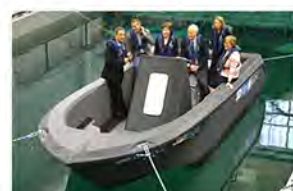
Case Study 4: 25' 3Drigo U. Maine Advanced Structures & Composites Center. 2019. Single gantry wide bead thermoplastic composite extruder. Extruded thermoplastic deep vee patrol boat.
