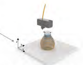
Additive Manufacturing: Common 3d Printing. FFF Method. Translates geometry into laminar toolpaths. Profile slices are deposited using XY coordinates. Easy to produce a variety of shapes and forms.
