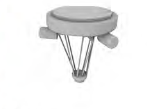
Parallel Robot Six Degrees of Freedom. Limited workspace. Used for high resolution prototyping fine positioning.
