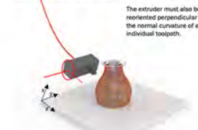
Extruder Orientation: Stronger surfaces w/ more layers. MBP Method. This is a second technical research challenge. Surfaces can be built with multiple layers to strengthen 3d form. The extruder is re-oriented to follow the geometry of surfaces.
