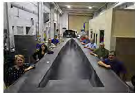
Case Study 3: 25' Catamaran demonstration project Oak Ridge National Laboratory MFD. 2019. Single gantry BAAM with 6-axis robotic mill. Extruded thermoplastic and finish-milled cavity mould.
