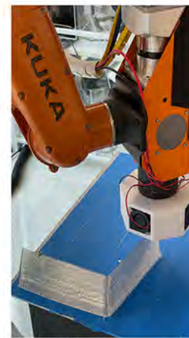
Assembly Testing MDPE2: Extruder with manual switch panel and Pointloader. Toolpath 1 laminar 1mm vertical offset parallel to World XY. Toolpath follows standard 3d printing logic.
