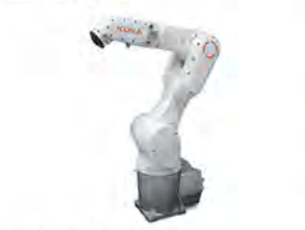
6-Axis Robotic Arm Six Degrees of Freedom. Moderate workspace and payload. Used for high-dexterity operations.
