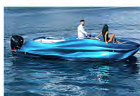
Case Study 6: 21' MAMBO motorboat. Politecnico di Milano, MOI Composites. 2020. Robotic arm CFM with FRP hand lay-up. Extruded continuous glass FRP motorized catamaran.
