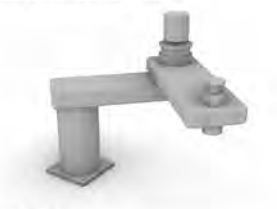
SCARA Robot Radial Coordinate System. Moderate workspace. Used for material handling and simple repetitive operations.
