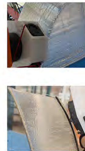
Assembly Testing MDPE2: Extruder with manual switch panel and Pointloader. Toolpath 2 vertical curves perpendicular to surface normals. Demonstrates MBAM logic for solid multi-layer surfaces (hull).
