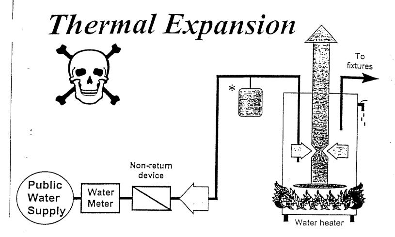
With "non-return devices" installed in domestic water piping systems, thermally expanded water is prevented from flowing back into the public water supply. The result is a "closed domestic water system" in which dangerous pressure increases may cause flue collapse, flame roll out, plumbing fixtures and the water heater relief valve to leak, and Carbon Monoxide.
