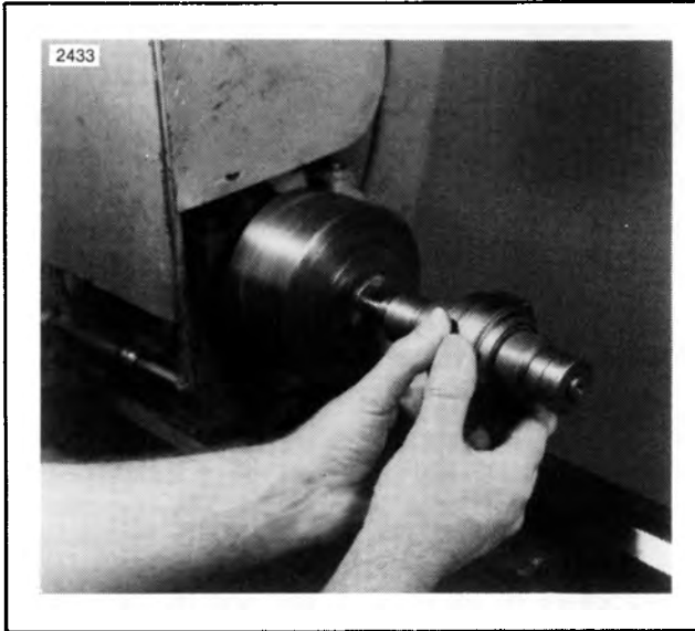
Figure 3-52. Lapping Connecting Rod
