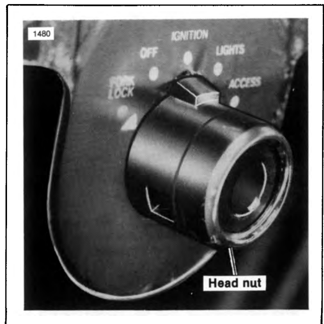
Figure 2-117. Ignition Switch Housing Head Nut
