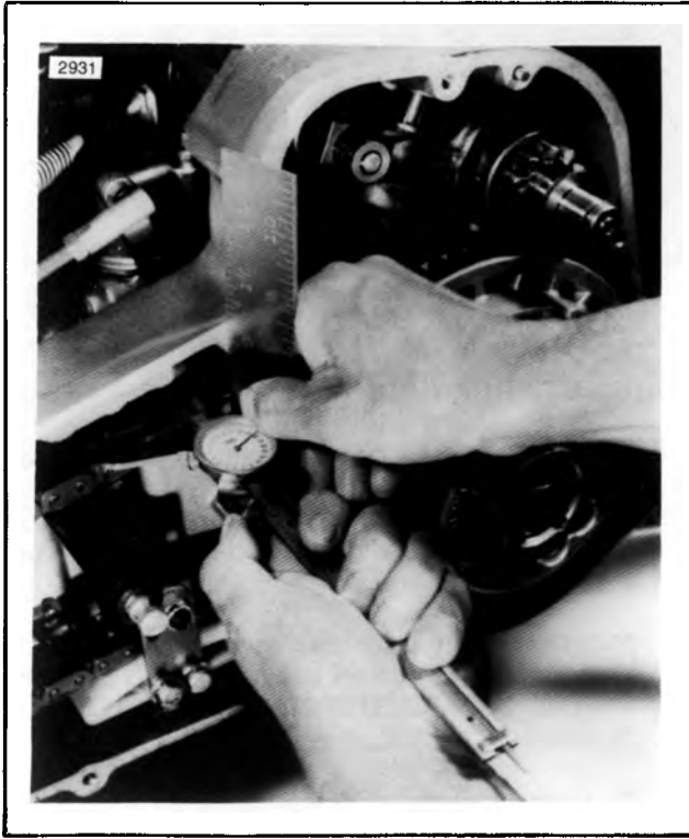
Figure 6-4. Checking Chain Alignment
