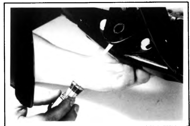
Figure 2-40. Aligning Mount Front-to-Rear
