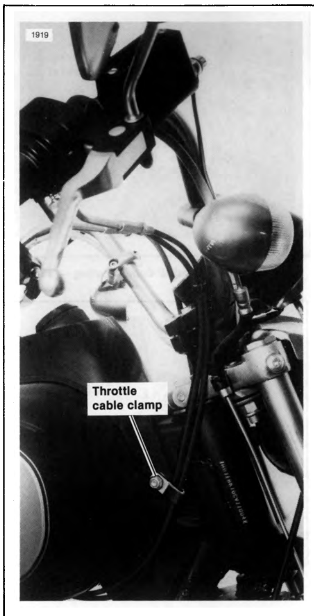
Figure 2-95. Throttle Cable Routing — FXR
