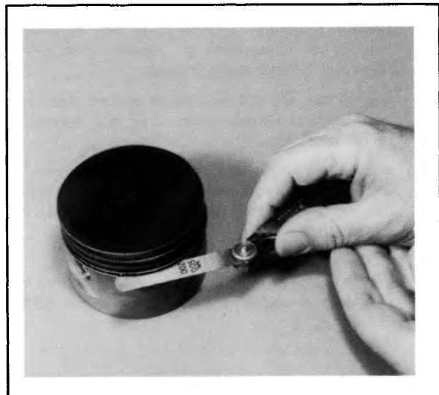
Figure 3-24. Measuring Ring Side Clearance
