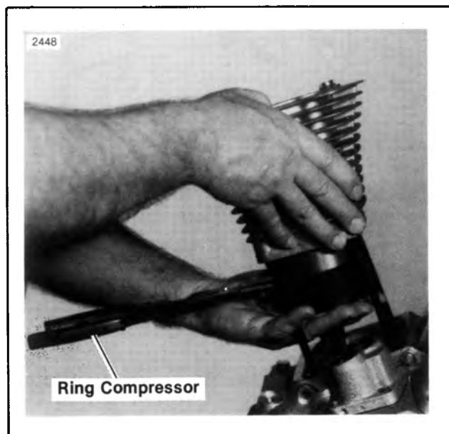
Figure 3-26. Slipping Cylinder Over Piston
