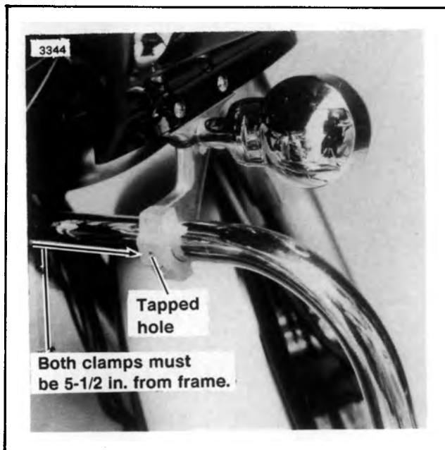
Figure 2-146. Upper Mount Location for Fairing Lowers
