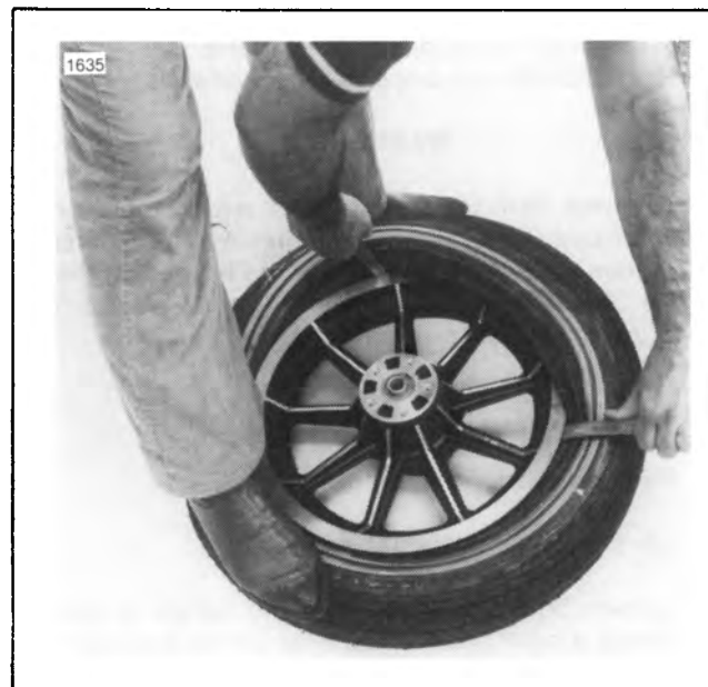
Figure 2-29. Starting Bead on Rim
