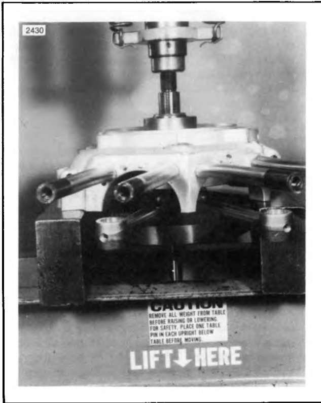
Figure 3-43. Pressing Flywheels Out of Crankcase
