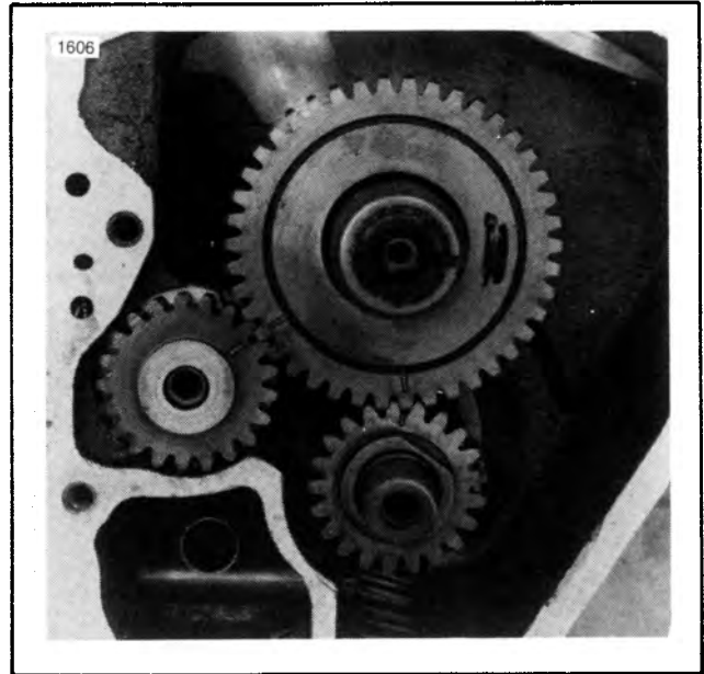
Figure 3-39. Timing Gears with Marks Aligned
