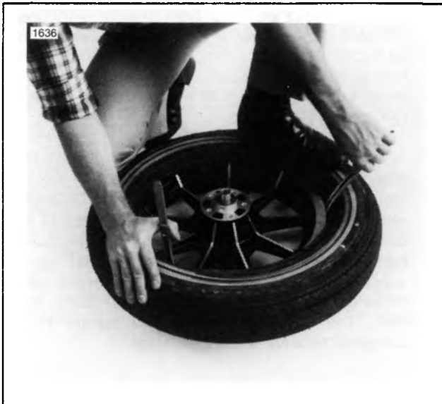
Figure 2-30. Starting Second Bead on Rim
