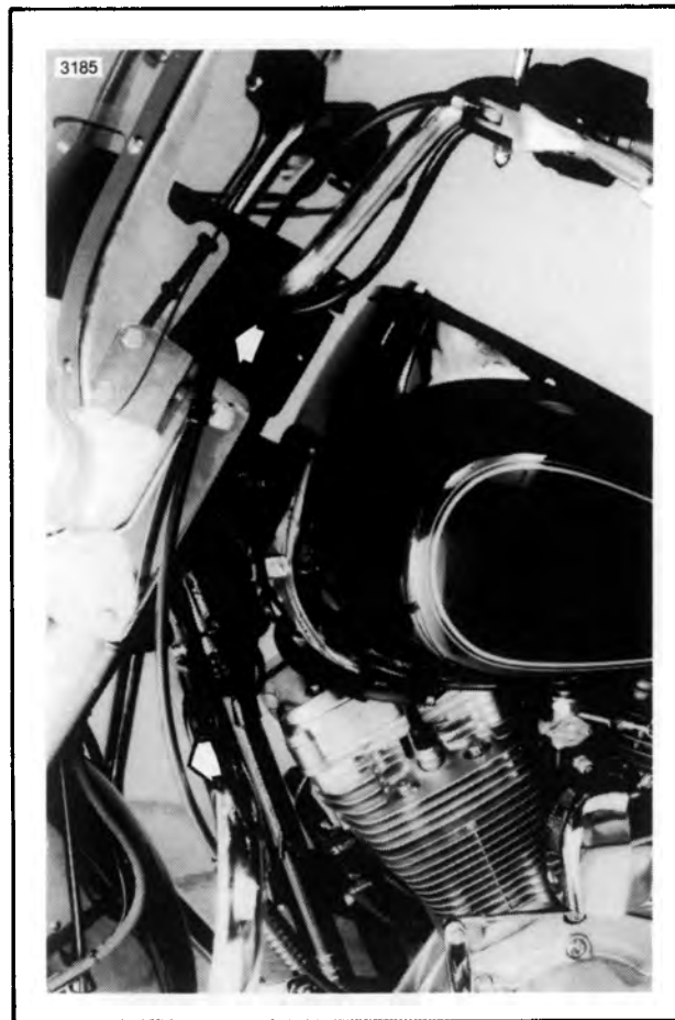
Figure 2-105. Clutch Cable Routing — FLHS
