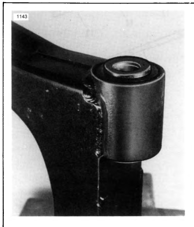
Figure 2-81. Clevebloc in Swing Arm
