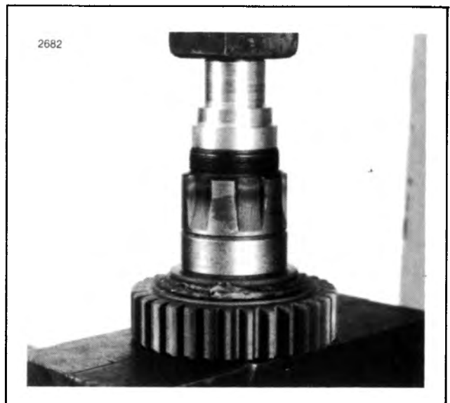
Figure 7-28. Pressing in Seal
