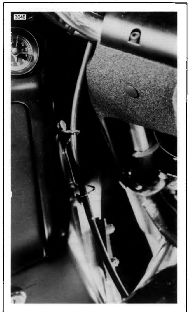
Figure 2-103. Clutch Cable Routing — 1987 FLT and Later
