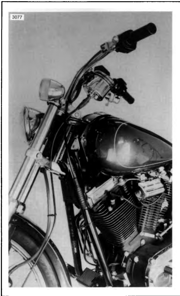
Figure 2-101. FXR Clutch Cable Routing — Left Side, 1987 and Later
