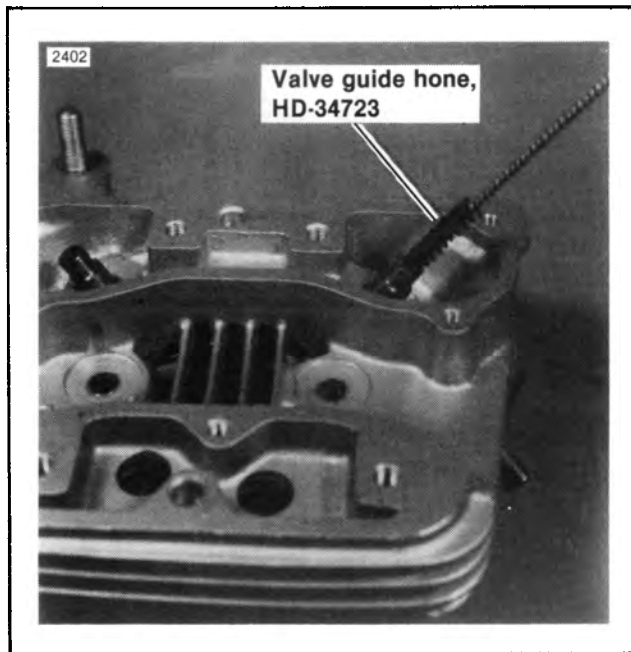
Figure 3-11. Honing Valve Guides
